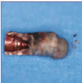
FIGURE 2 Fractured implant removed
